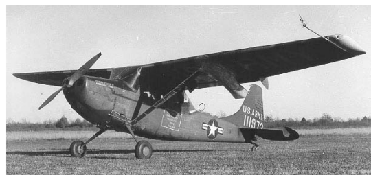
Fig. 34 L-19 observation aircraft with boundary-layer control.
