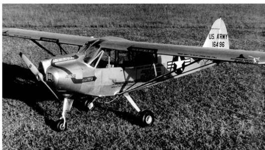
Fig. 29 L-21 observation aircraft used for boundary-layer control studies.
