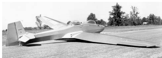
Fig. 22 Schweitzer TG-3A used for boundary-layer separation studies.
